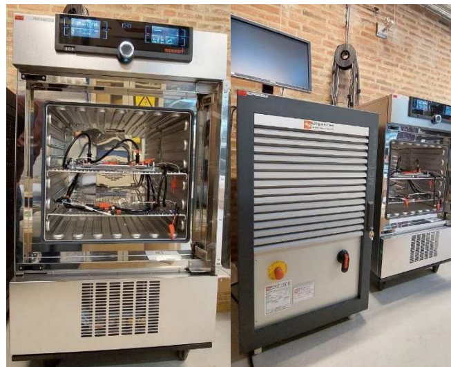
Fig. 1. Battery test setup. Digatron BTS 600 (right), Memmert UFP 600 temperature chamber containing LIC battery(left).
