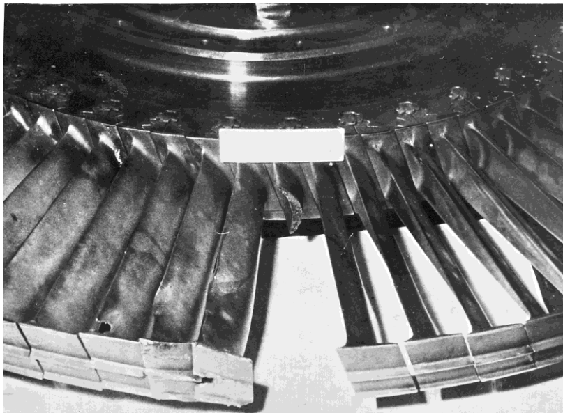
Fig. 7. Weakening of bandage connections due to creep in thin peripheral sections and breakage of a blade under the action of thermomechanical and vibrational stresses
