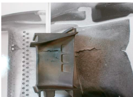
Fig. 1. Localization of HPT nozzle blades damages in a zone of maximum temperatures action (in 1...2 mm spots)
