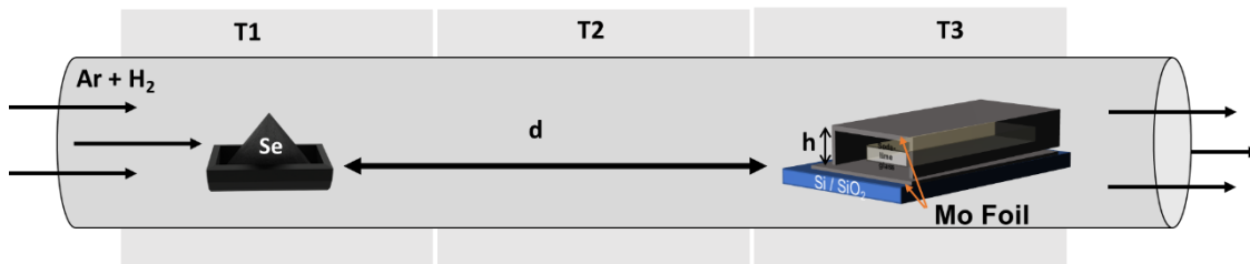
Figure 41. Schematic illustration of the experimental setup utilized for the synthesis of MoSe 2 .
