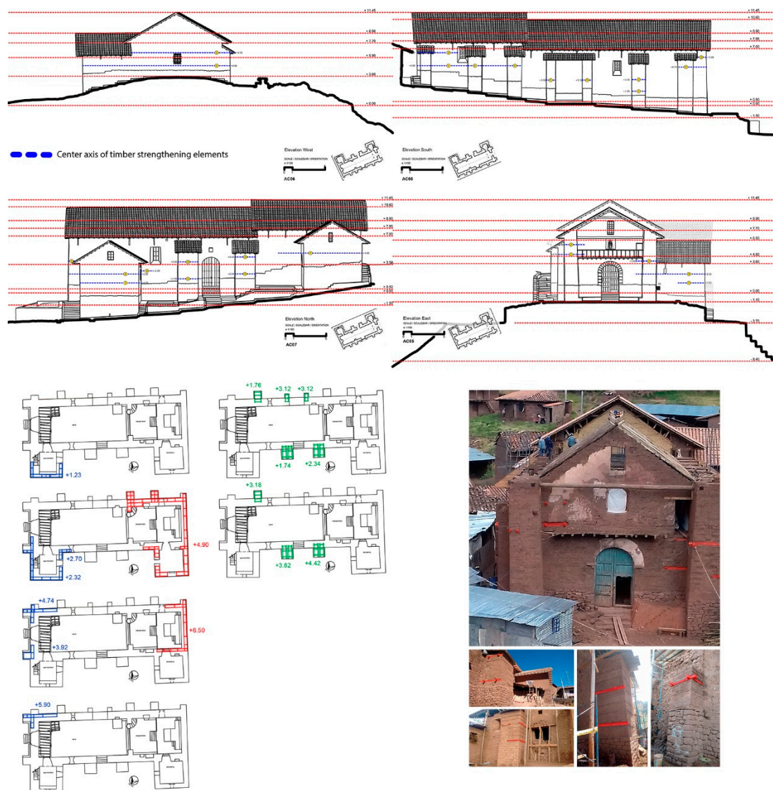
Figure 4. Configuration of timber-embedded corner keys and horizontal buttress timber keys in elevation. Several views are shown during the retrofitting work, with the timber-embedded elements highlighted in red.
