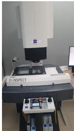
Figura 31- Máquina CMM multissensor zeiss o-inspect 322
