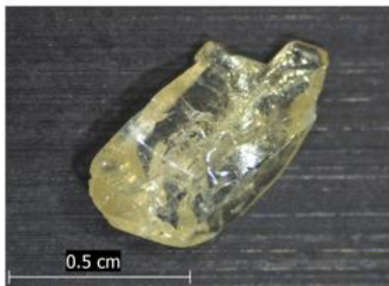
Figure A50. A solution-grown crystal of RInBr 4 .
