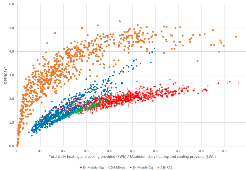
Figure 6 Daily heating and cooling performance factor for system boundary 5 (DPFHC5+) against daily heating and cooling loads normalized by the maximum daily heating and cooling loads for each system.
