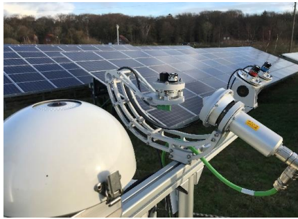
Figure 2: Instrumentation installed in a solar plant showing the ASI (left), the RSI (center) and the tilted pyranometers (right).
