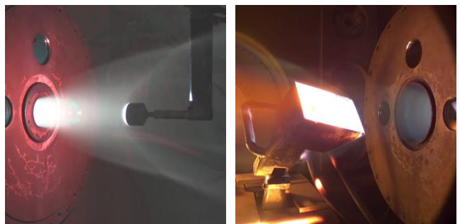
Figure 7: Stagnation (left) and tangential (right) setups during experimental entry flight simulations.
