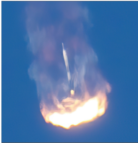
Figure 1: Image of a Falcon 9 first stage booster performing a three engine hypersonic retro-propulsion maneuver during atmospheric re-entry [3] (refer to [4] for video comparison)
