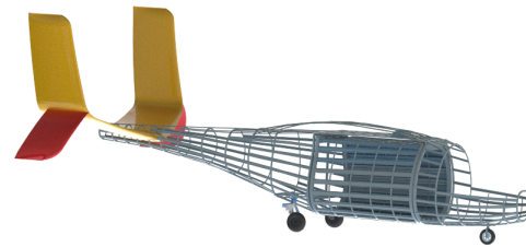
Figure 28 – Structural concept of fuselage with module installed
