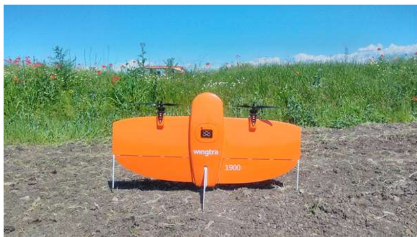
Fig. 4. WingtraOne UAV type wing used in the study
