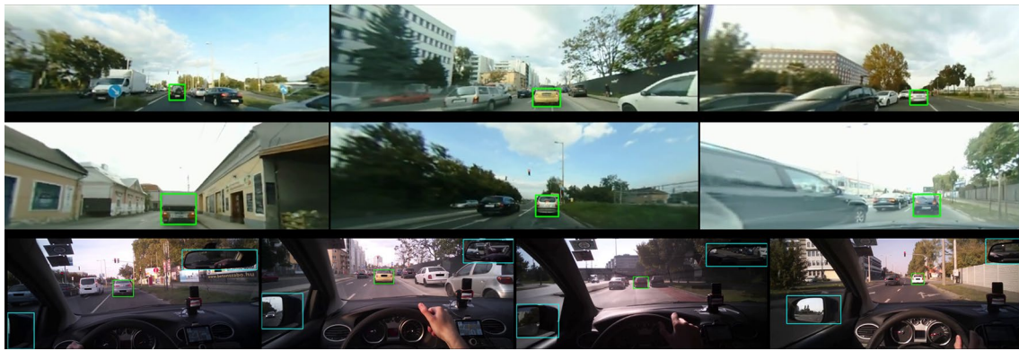
Fig. 1 Sample image frames from our self-collected driving videos. The first two rows present wide equirectangular projections extracted from the spherical videos, with the detected lead vehicle highlighted.
