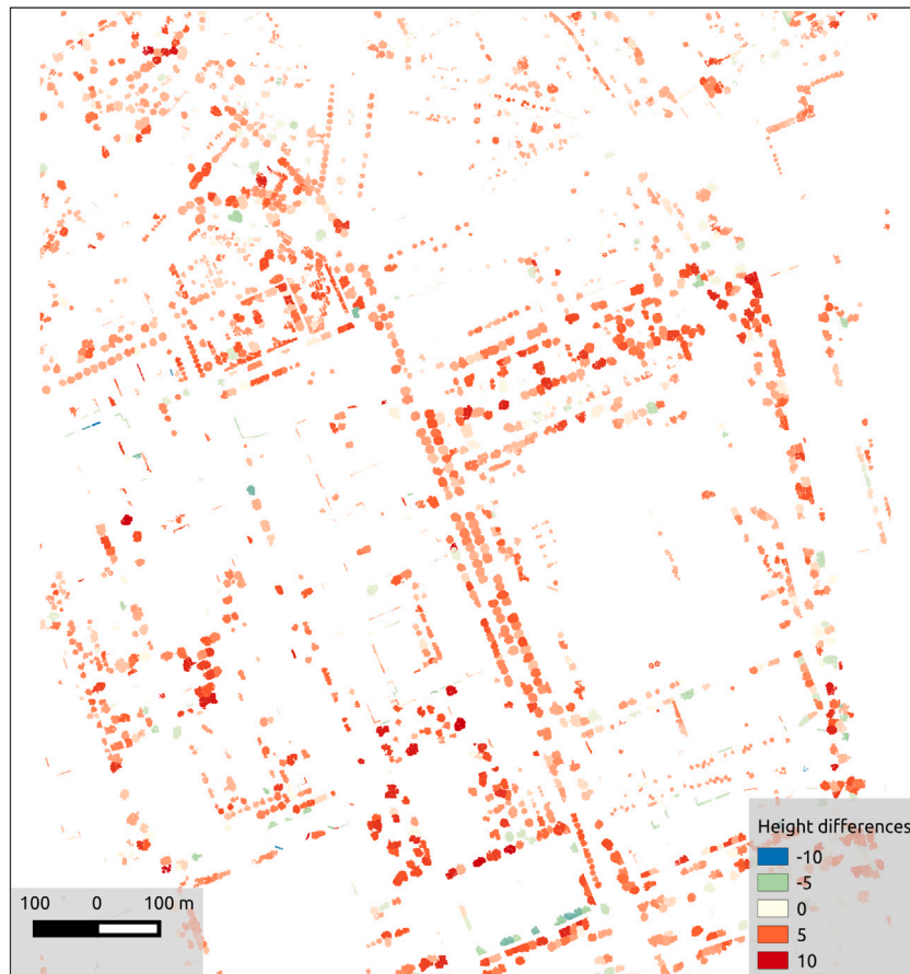
Fig. 12. Height differences of paired clusters in the TU Delft Campus sample territory.
