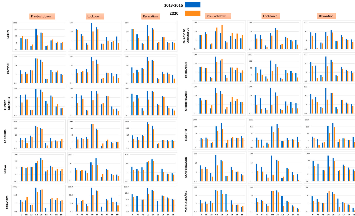
Fig. 4. Comparison between mean trace elements concentrations ( \text{ng m}^{-3} ) during 2020 and the period 2013–2016 taking into account the three different mobility periods: pre-lockdown, lockdown and relaxation.
