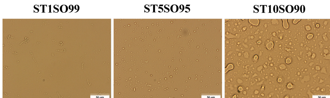
Fig. 9. Micrographs of stearic acid-in-silicone oil emulsions at 90 ^{\circ}\text{C} after heating-cooling cycles.
