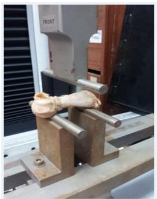
Figure 1: Test setup of the 3-point bending tests
