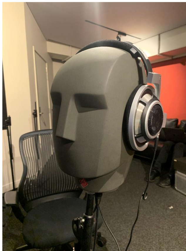
Figure 2-6 Neumann KU 100 Dummy Head system used for headphones calibration
