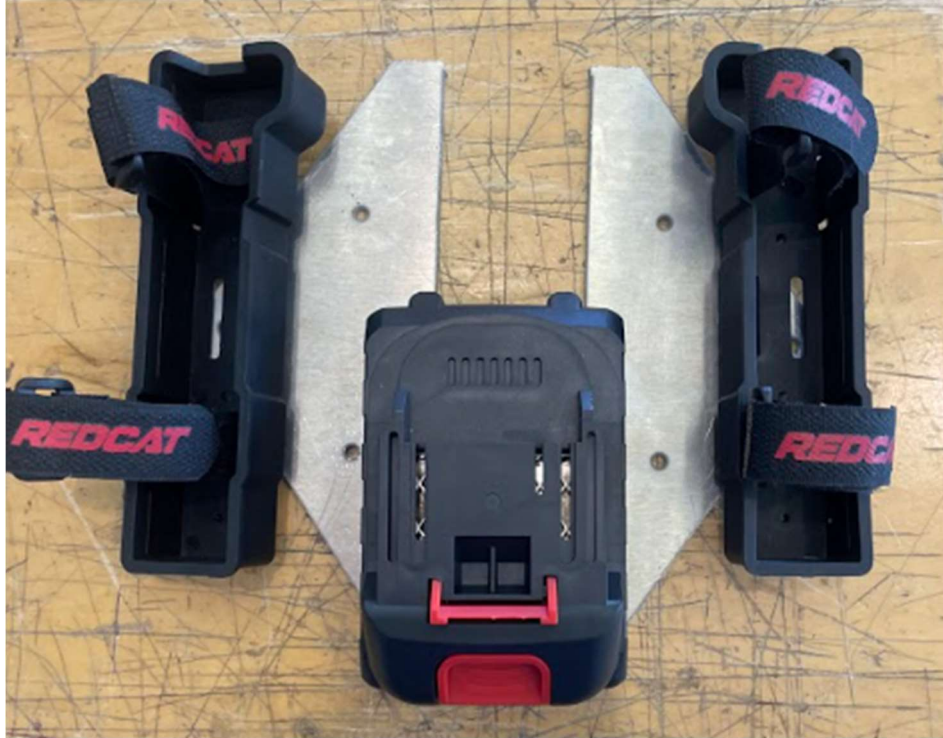
Figure 17. Car and Chainsaw Batteries Layout on Top Plate
