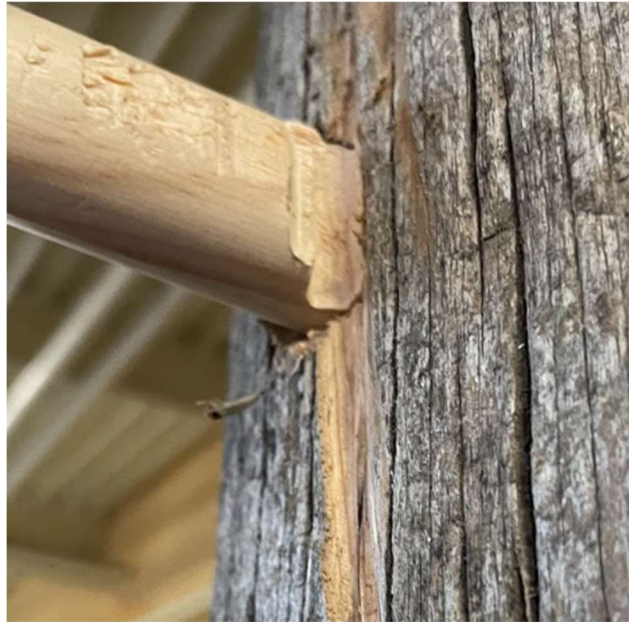
Figure 23. Results of Cutting Test with Chainsaw
