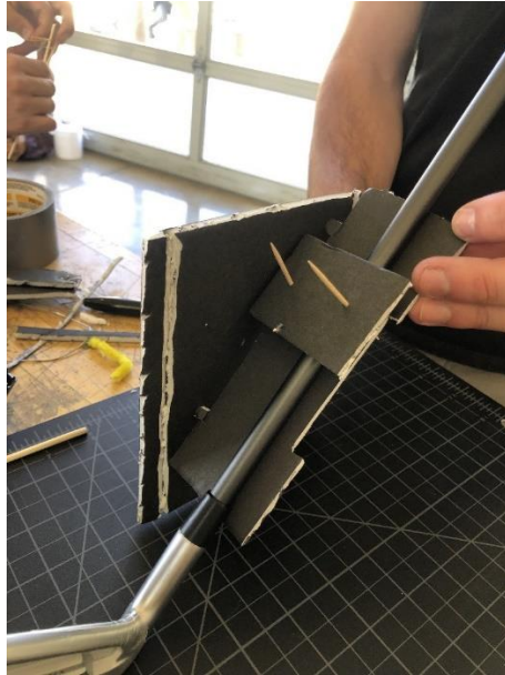
Figure 5: Clamping mechanism that tightens down with screws (represented with toothpicks) to securely hold mandrel or shaft in place. Loosen screws to change shaft or mandrel out or to adjust position of club.
