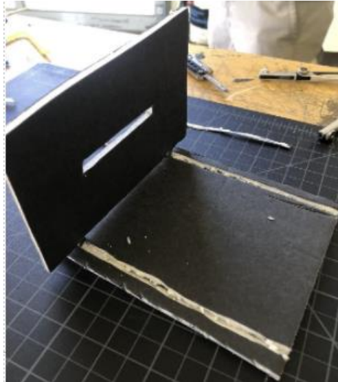
Figure 8: Track System that slides to contact the secured club face.
