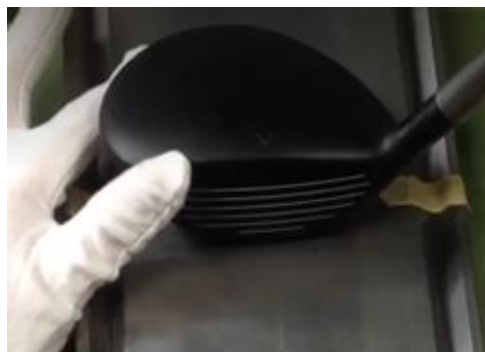
Figure 2.3: Rotating Club to Make First Point of Contact with Manufacturer's Keel Point Distance
