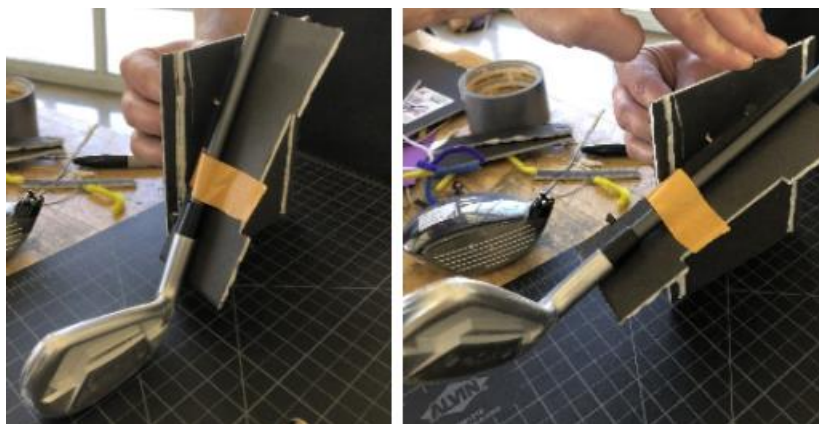
Figure 10: Rotating shaft connection for measuring lie angle.
