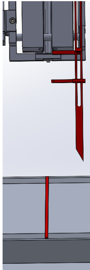
Figure 3.3A: Keel Point Slider zeros at shaft/mandrel centerline.
