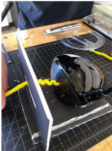
Figure 4: 4-point laser contact to establish distances for angle conversions of loft and face angle. The red dashed lines signify distances calculated using laser-distance technology. By measure from the reference plane on the left-hand side, the four measurements from the laser-distance scanner will define the measurements of the plane. From here, software can be used to calculate the face angle and loft of the clubhead. We really like this idea because this kind of measurement technology is versatile and can be used for every club. Furthermore, this technology already exists, so we would just need to figure out a way to extract the data and run calculations from it.
