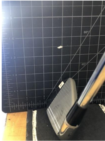
Figure 3: Setting the clubhead down on a flat datum and measuring the loft angle by putting a grid behind the clubhead and taking a picture. The grid is made up of squares and when photo is taken, the computer will calculate the slope made by the club and convert it to an angle from the Zenith. We think it is a good idea, but we think it may take a lot of research to figure out the correct way to make this solution feasible.
