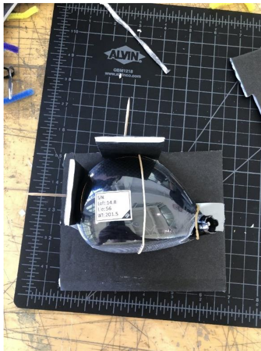
Figure 2: Sliding clamps to secure club head for purpose of central datum. Not seen is the shaft connected to the clubhead to secure it from a third location.
