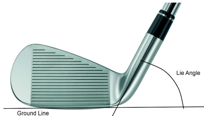
Figure 2: Visual depiction of the lie angle measurement (Kelley).
