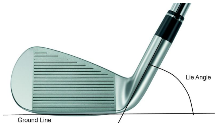
Figure 6: Visual Depiction of the Lie Angle Measurement [3].
