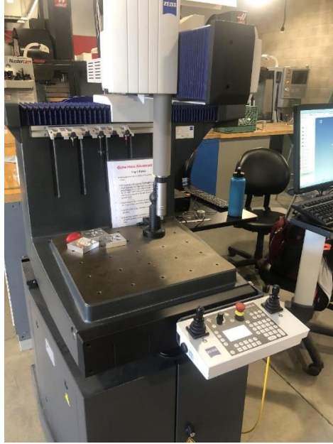
Figure 3: Coordinate Measuring machine.
