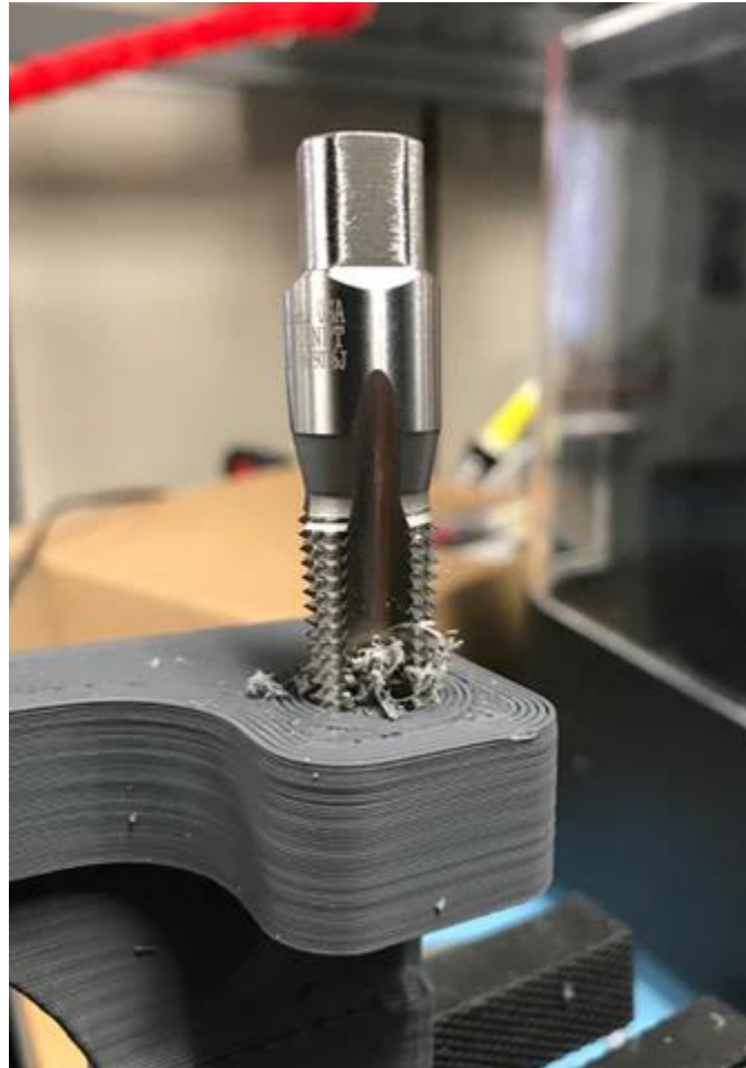
Figure 2.4: Tapping a 3D Printed Part
