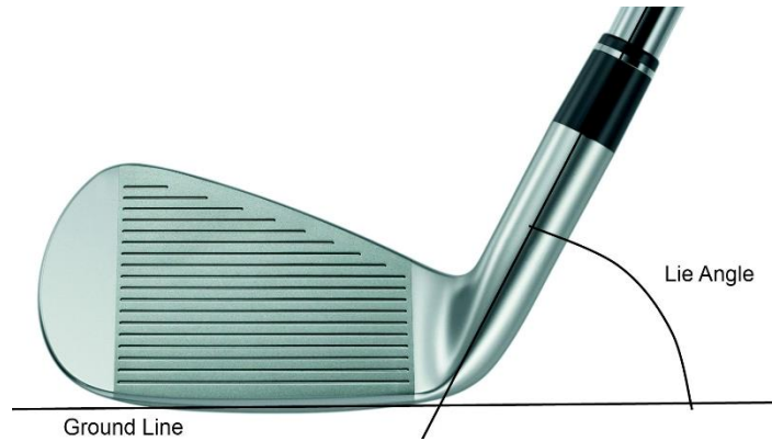
Figure 2.6: Visual Depiction of the Lie Angle Measurement [3].
