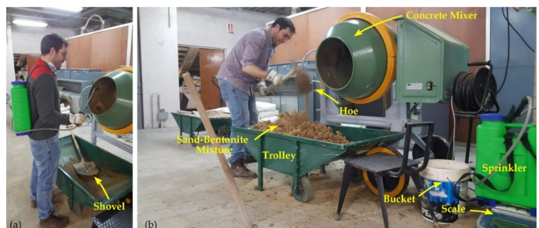
Figure 2. Images of the mixing process: (a) Sprinkling the sand-bentonite mixture with water while the concrete mixer is working; (b) Final moisture homogenization using a hoe.
