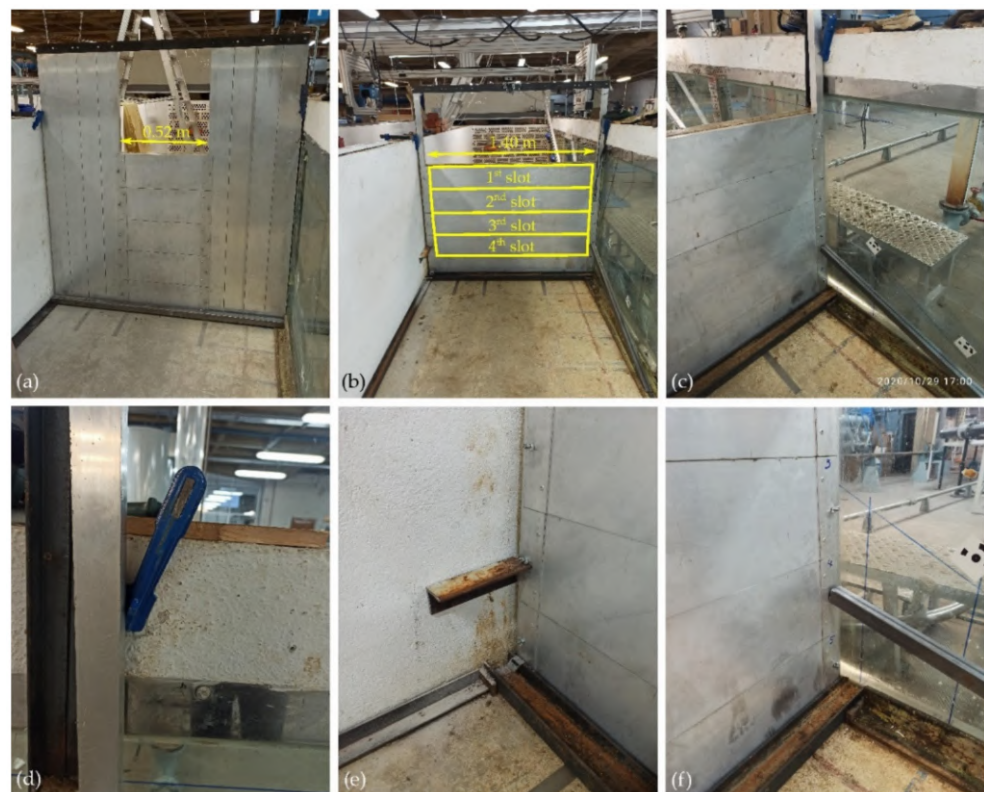
Figure 4. Images of the aluminum protection system for the simulation of the support of the core on the downstream shoulder: (a) Smaller unprotection width; (b) Larger unprotection width; (c) Detail of the '1/3' height metallic supports on the left wall of the flume; (d) Detail of the clamps used to support the upper section; (e) Detail of the metallic supports on the right wall of the flume; (f) Detail of the metallic supports on the left wall of the flume.
