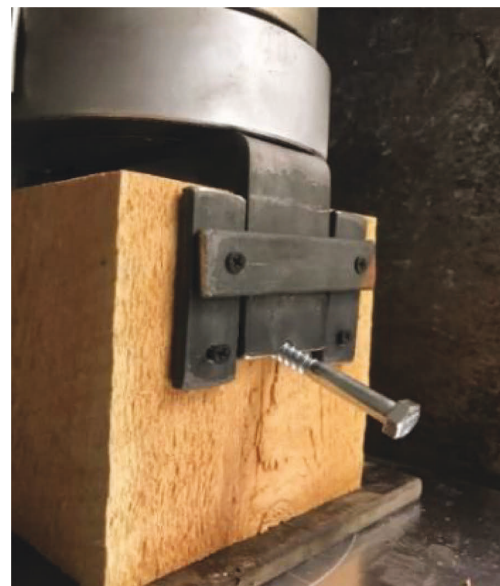
FIGURE 6: Lag screw yielding at 6.6 cm.
