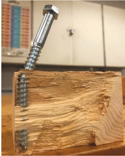
FIGURE 7: Lag screw section at 6.6 cm embedment.
