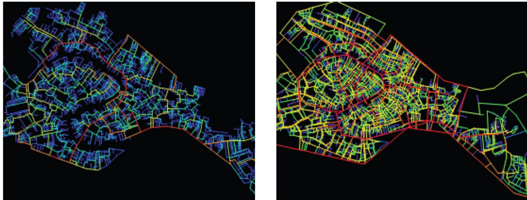
Figure 1: Space Syntax Angular Segment Analysis of Venice without (left) and with (right) canals (Source: Hillier, B. (2016) 'What are cities for? And how does this relate to their spatial form?', Journal of Space Syntax , 6(2), pp. 199–212.)
