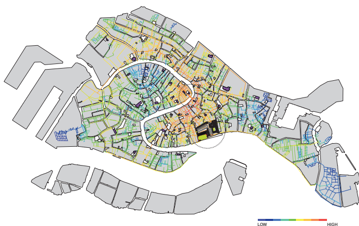
Integration values of pedestrian network in Venice. Integrated spaces are easy to reach from every other space in a layout, constituting the spaces where movement paths converge. In contrast, segregated spaces can be accessed through paths that involve many changes of direction, expressing status or social difference – Plan: S. Psarra, 2018.
