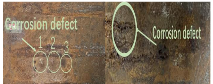
Fig. 12 natural corrosion pits and natural corrosion cracks.
