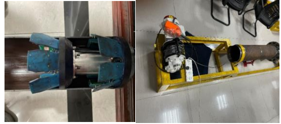
Fig. 10 (a) Smart pigging, (b) the detection system for pipeline defects.
