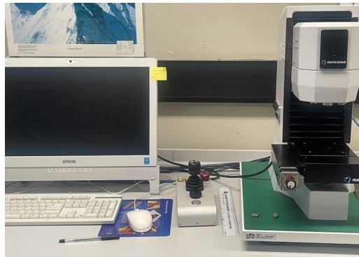
Fig. 3.15 Matsuzawa Via-F automatic Vickers tester
