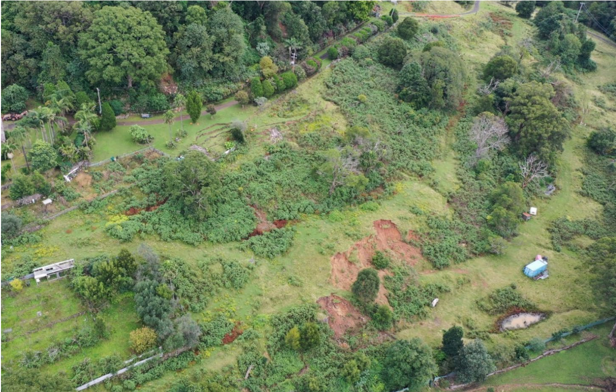
Figure 5. This site is immediately north of the area shown in Figure 4. Several walkover inspections of this site with a Trimble Geo 7X has identified a large slide category landslide with an area of 16,500m 2 and with an assumed maximum depth of 7m, a volume of approximately 70,000m 3 . RPA photo by Flentje.
