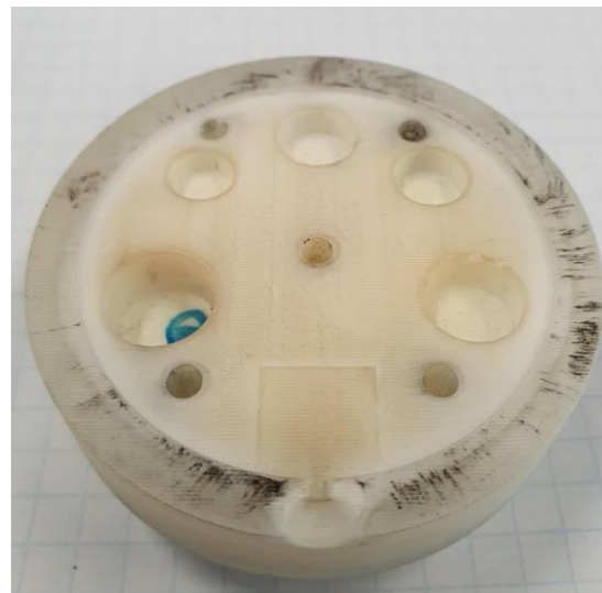
Figure 21. 3DIM cavity showing no signs of deterioration after 10 moulding shots.
