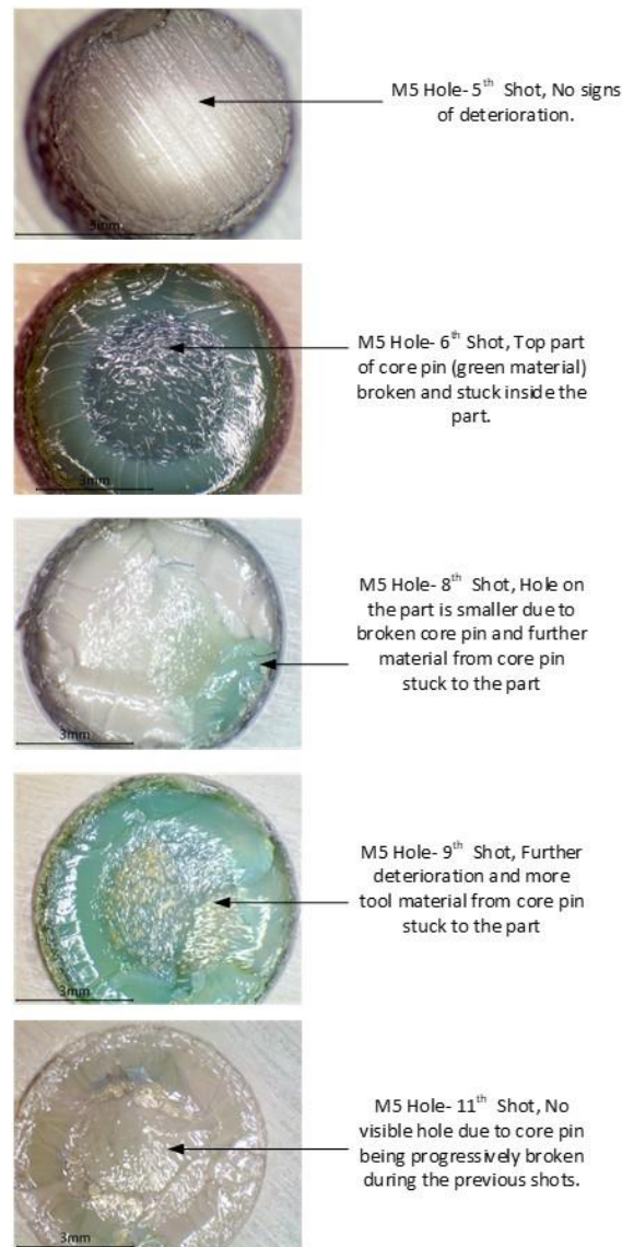
Figure 23. Progressive reduction in depth of the M5 core hole as a result of deterioration of the M5 core pin. (The green material is the core pin that been chipped and stuck onto the part during ejection).
