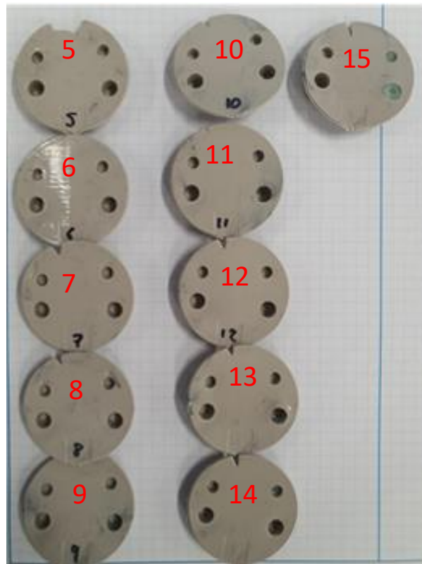
Figure 25. Part sequence, moulded using 20 s cooling time. Numbers refer to shot. Parts 1–4 not shown as they were not fully formed due to shorter cooling time. Mould failure occurred at shot 14.
