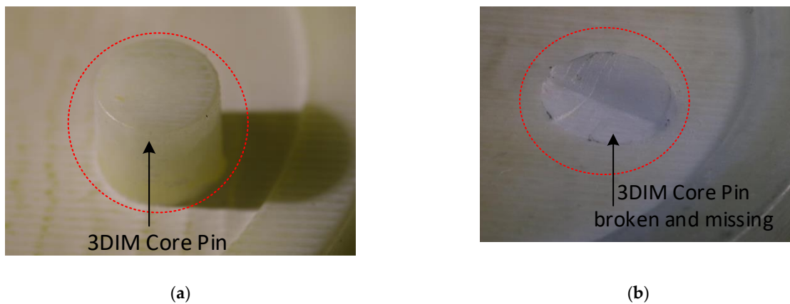
Figure 19. (a) 3DIM tool with an intact core pin before moulding; (b) 3DIM tool with a broken a missing core pin after moulding and part ejection during 3rd shot.
