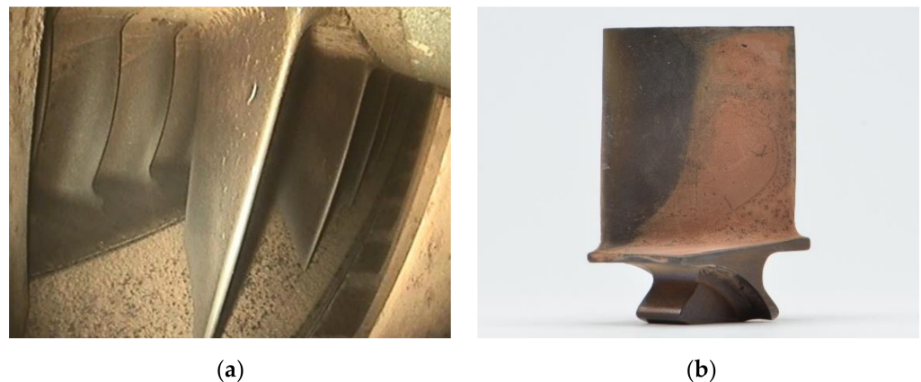
Figure 1. Two types of engine blade inspections: (a) in-situ borescope inspection, (b) on-bench piece-part inspection.
