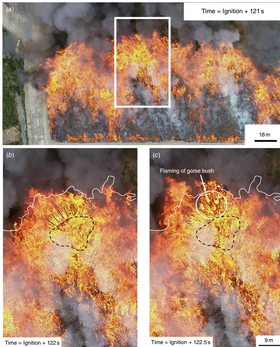
Fig. 4. Observed flaming zone in plot P2 from nearly 200 m AGL using a UAV. Panels (b) and (c) cover the spatial area outlined in the white box in panel (a). The white lines in panels (b) and (c) represent the flame front at time of ignition plus 121.5 s. The black dotted outline in (b) and (c) shows the area of a fire 'sweep' and its impact on vegetation ignition. The black radial lines from panel (b) represent the direction of the flames emanating from the circumference of the fire sweep.
