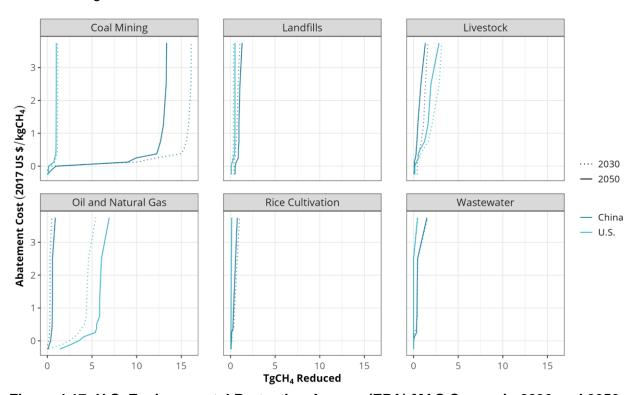
Figure 4.17: U.S. Environmental Protection Agency (EPA) MAC Curves in 2030 and 2050 in the U.S. and China (EPA, 2019b). The U.S. EPA MAC curve was used in the GCAM model to project emissions reduction potential.
