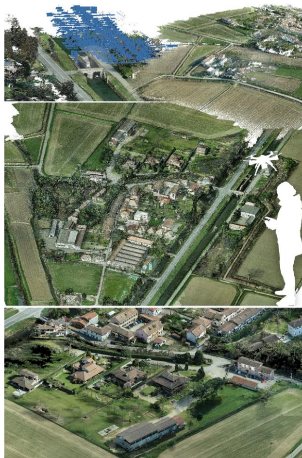
Figure 2. Geometric and morphological documentation was conducted by fast-survey techniques using UAV tools with Structure from Motion close-range photogrammetry.
