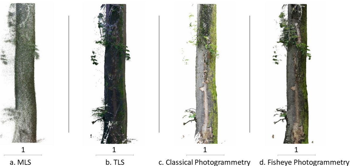
Figure 2. Transversal section of tree stem acquired by terrestrial remote sensing methods. Scale bar units are in meters.
