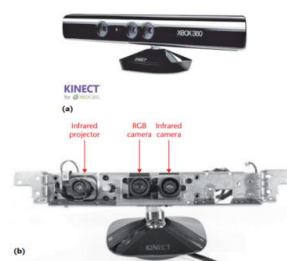
Figure 2. Kinect 2.0 sensor parts
