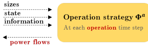
Figure 1.4: The operation strategy gives, at each operation time step, the power flows as a function of the available information and state of the system.
