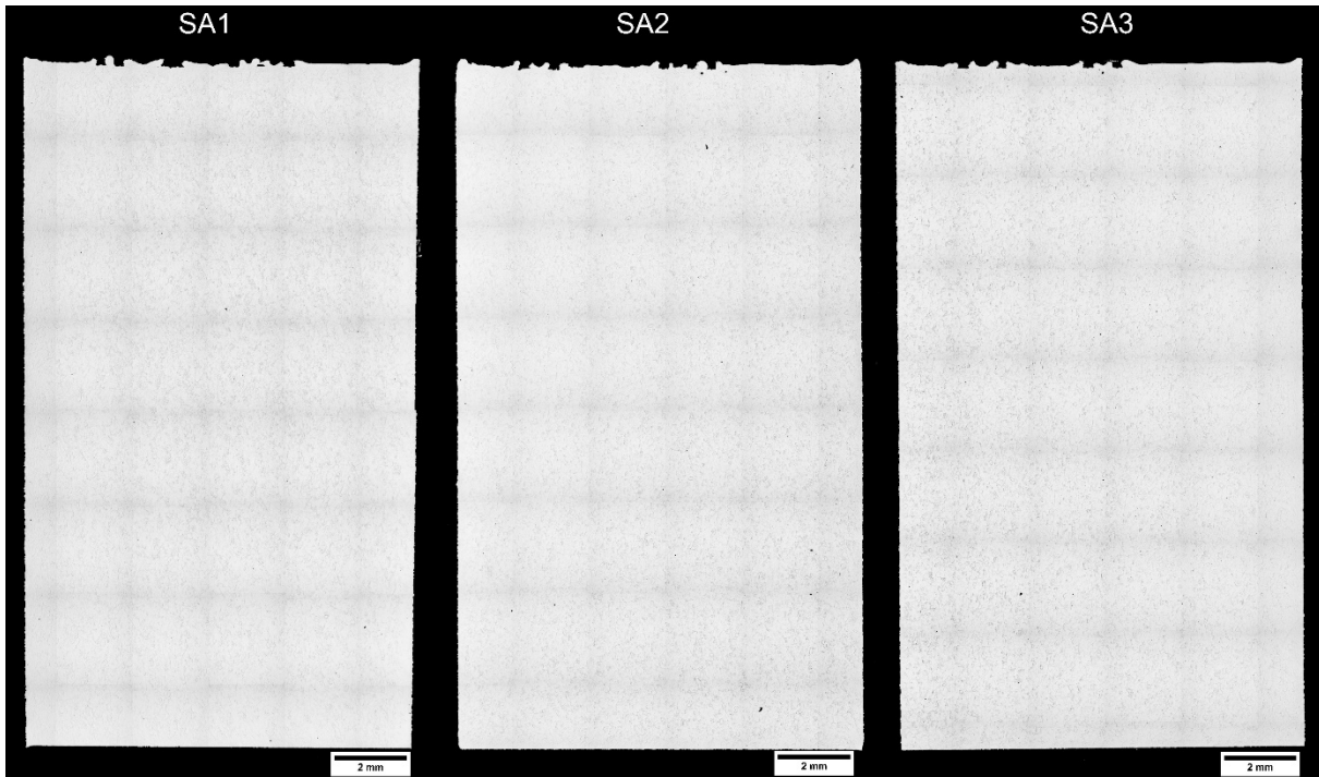
Figure 4. OM images of polished cross-sections used for porosity analysis
