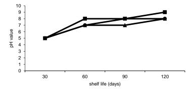
Figure 1. The results of the pH value test of the defect tanned leather solution during the shelflife. The defect tanned leather pickle (square). The defect tanned leather wet blue (round), The defective upper shoe leather (Triangle).
