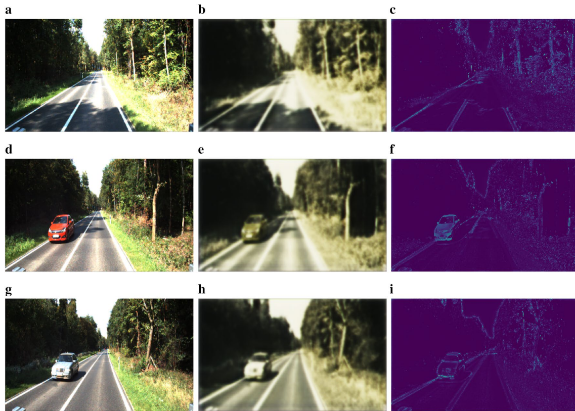
Fig. 6 Autoencoder visual example results for KITTI dataset: a input image for the normal driving scenario (empty road), b reconstructed image for the normal driving scenario (empty road), c reconstruction error image for the normal driving scenario (empty road), d input image for the anomalous driving scenario (red car), e reconstructed image for the anomalous driving scenario (red car), f
