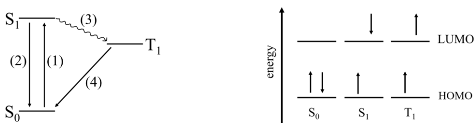
Scheme 4. (Left) Simplified Jablonski diagram with ( S_0 ) ground singlet, ( S_1 ) excited singlet, and ( T_1 ) excited triplet electronic energy levels and the transitions between them; (1) absorption, (2) fluorescence, (3) intersystem crossing, and (4) phosphorescence. (Right) Diagram showing how electronic spin and energy level determine ( S_0 ) ground state singlet states, ( S_1 ) excited singlet states, and ( T_1 ) excited triplet states.
