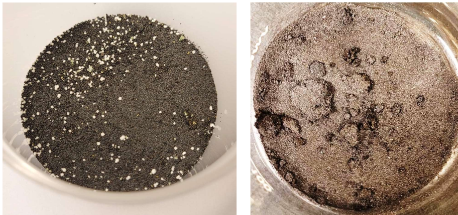
Figure 18: Photos of samples collected after the experiments with the addition of K_2CO_3 . Left: the sample from the experiment at 850°C showing the presence of white grains. Right: the sample from the experiment at 950°C showing lumps of agglomerated particles.
