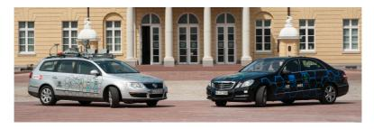
Figure 6.1.: Experimental vehicles of the Institute of Measurement and Control Systems. AnnieWay (left) used in the DARPA Urban Challenge [80] and BerthaOne (right) used in preparation of the Bertha Benz Memorial Drive [184].
