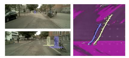
Figure 6.8.: Trajectory optimization: from labels in images (left), initial position estimates are created (right, triangles). These are then optimized for ground-truth-like trajectories (right, solid lines). Note: the gray blobs at the lower end of the optimized trajectories are measurements of the two pedestrians accumulated in the grid.
