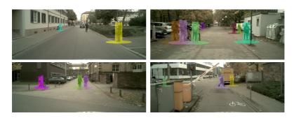
Figure 6.7.: Pedestrians annotations in images. Information includes the enclosing bounding box, position w.r.t. the vehicle and occlusion.
