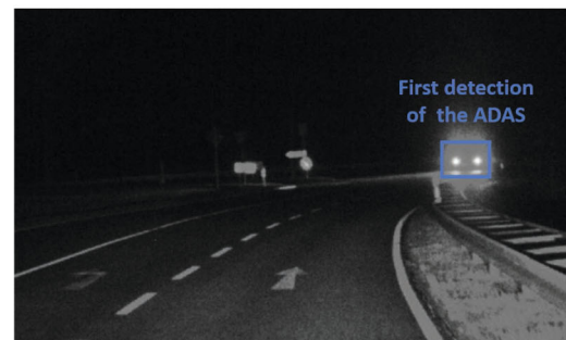
(d) First detection of the in-production system based on direct light instances 3.8 s after first sight.
