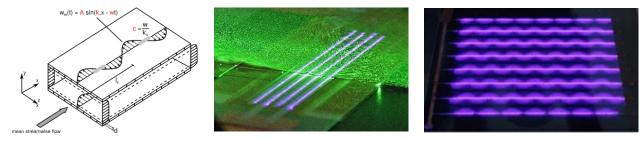
Figure 1: StTW of spanwise wall velocity. (a) Duct section and wall-velocity profile w(x) of StTW. Reproduced from [6]. Spanwise forcing in (b) for virtual wall oscillation [10,11] and in (c) for (streamwise) standing waves [12] of virtual spanwise wall velocity.
