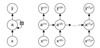
Figure 2.3.: RNN in a folded (left) and unfolded (right) state. Grey square indicates time step delay
