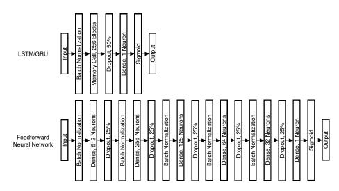
Figure 2.2.: Architecture of applied feedforward neural networks (bottom) and recurrent neural networks (top). Note: For the recurrent networks, the memory cell is either an LSTM cell or a GRU cell
