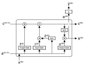
Figure 2.4.: LSTM memory block with input, forget, and output gate (based on Olah 2015)
