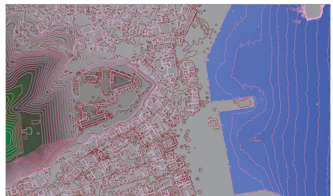
Fig. 5. Comparison of topographic data between laser scan and STL (red broken line: laser scan; and pink solid line: STL).
