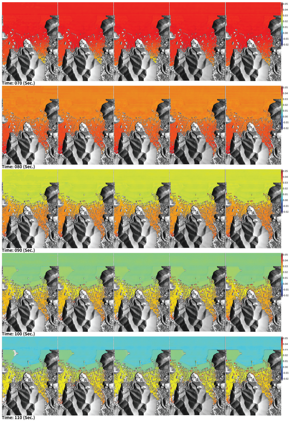
Fig. 12. Time series of spatial water level for the case of long period wave ( t = 70\text{--}110 s; code name from the left to right: I, NK, TN, JT, and JM).
