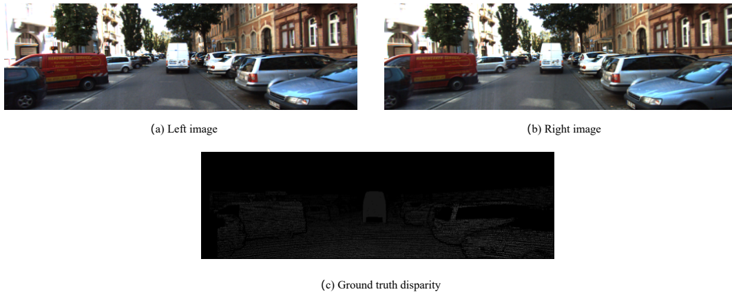
FIGURE 3.5: KITTI 2015 dataset. (a) left image of stereo image pair, (b) right image of stereo image pair, (c) ground truth disparity.
