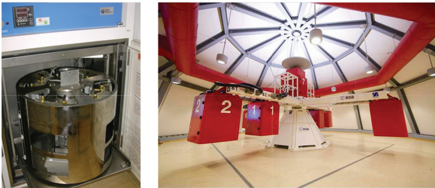
Figure 11.1 Two examples of research centrifuges. Left The medium-diameter centrifuge for artificial gravity research (MidiCAR) is a 40-cm-radius system for (mainly) cell biology research [16]. Right The large-diameter centrifuge (LDC) [6] is an 8-meter-diameter system used for life and physical sciences and technological studies. Both centrifuges are located at the TEC-MMG Lab at ESA-ESTEC, Noordwijk, The Netherlands.
