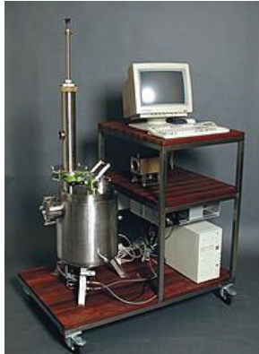
Figure 5.1 The Mars environmental simulation chamber. Image credit Mars Simulation Laboratory, Aarhus University.
