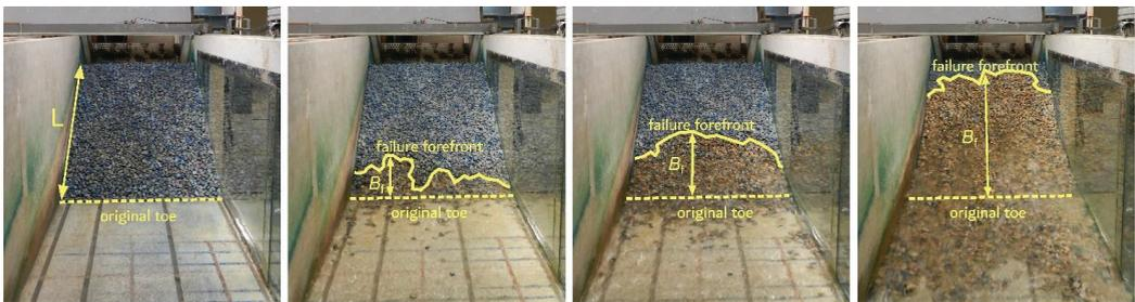
**Figure 2.** Scheme of the failure process sequence for discharges of  $0, 0.0188, 0.0256,$  and  $0.0423 \text{ m}^3 \text{ s}^{-1}$  (test n° 133,  $H = 1 \text{ m}, W = 1.32 \text{ m}, Z_{dss} = 1.6,$  gravel M7).
