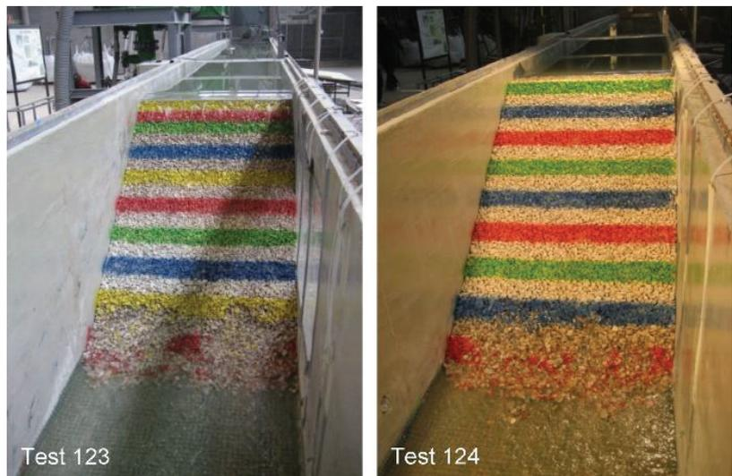
**Figure 17.** Failure progress in tests n<sup>o</sup> 123 and 124 for a discharge of roughly 0.0090 m<sup>3</sup> s<sup>-1</sup>.
