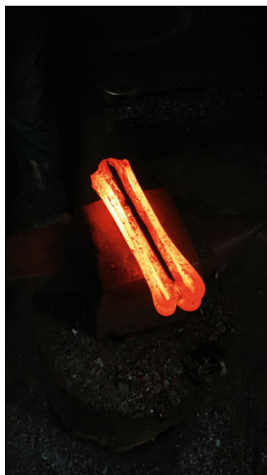
Fig. 7.26 The three-layer composite steel that was used for forging the blade
