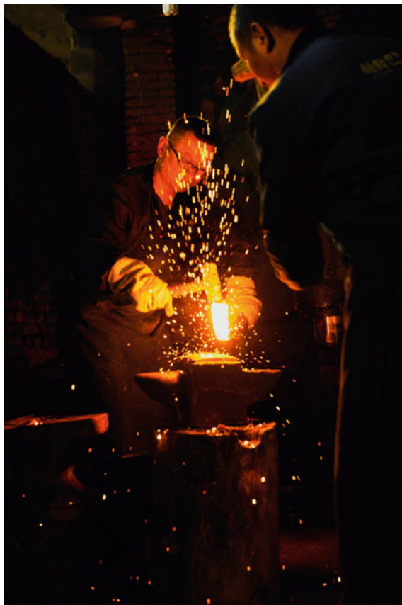
Fig. 7.22 Fold, stack, and hot forge the steel repeatedly with traditional methods to remove impurities from steel
