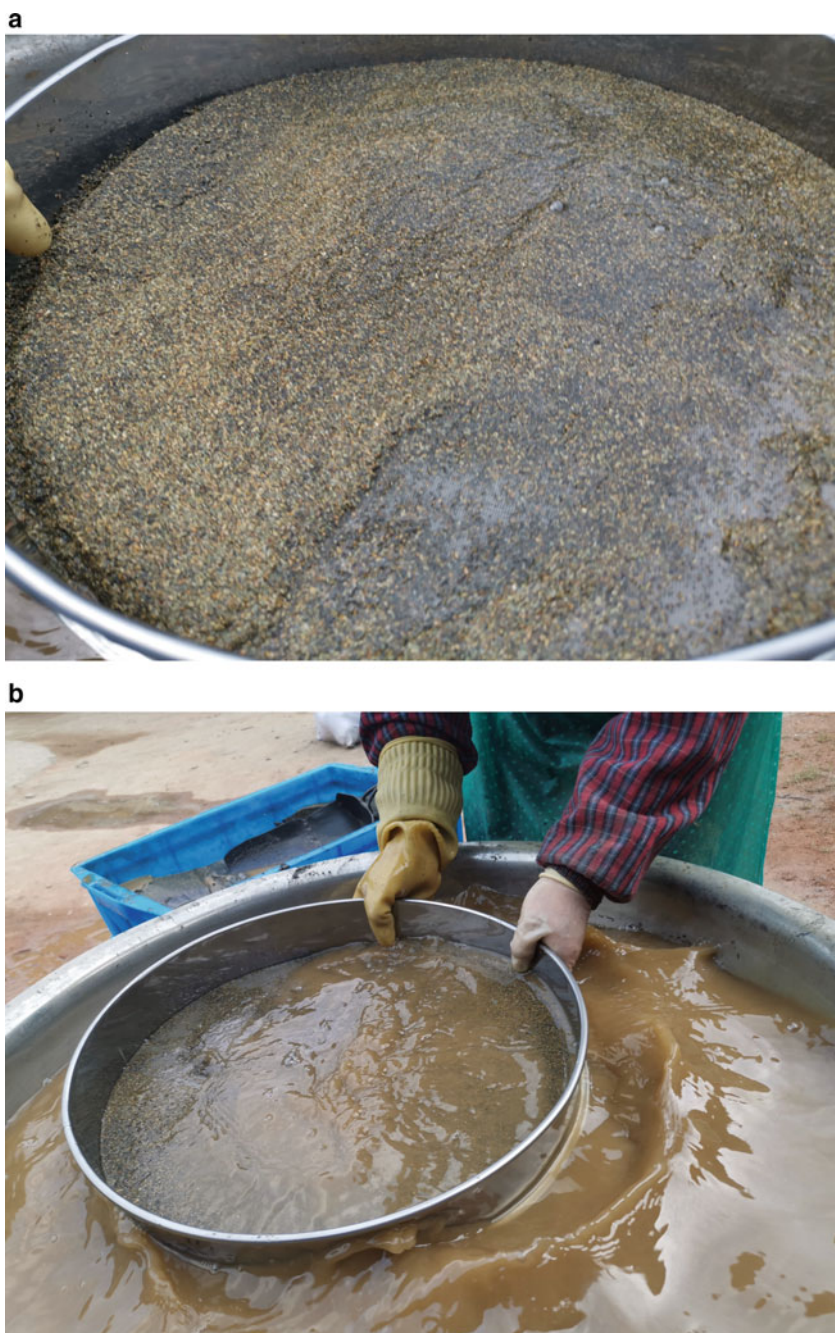
Fig. 7.3 Wash high-grade iron sand from the Ou river, Longquan, to remove impurities
