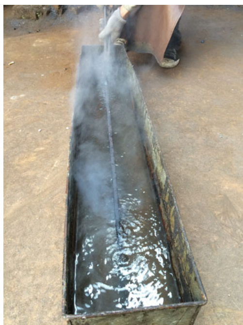
Fig. 7.31 Quench the blade in water
