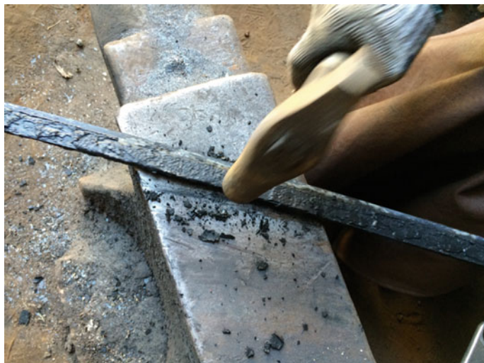
Fig. 7.32 Coldwork the blade to adjust its shape
