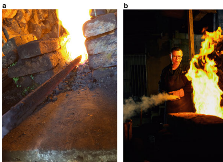
Fig. 7.30 Heating the blade before quenching
