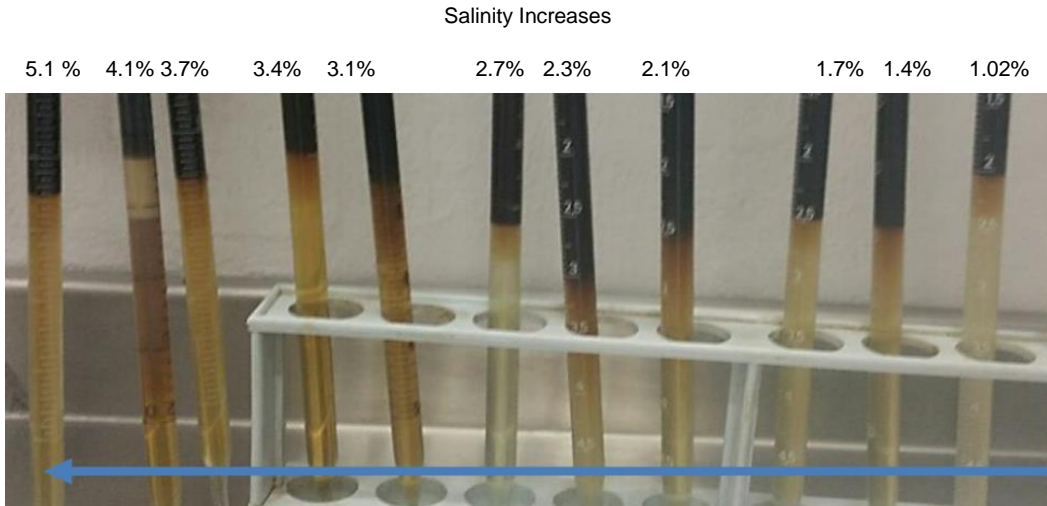
Figure 5-29: Phase separation test for surfactants ( C_{13-14} —7APS + C_{06-10} -AES) at 140 °F
